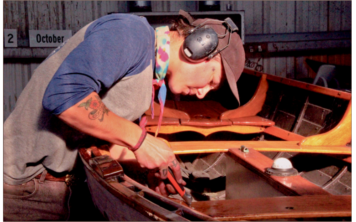
Lou Geraghty peels away old varnish as part of a refinishing job on the beautiful dinghy Loki , the first indoor job assigned to Horus Horizon Marine.
