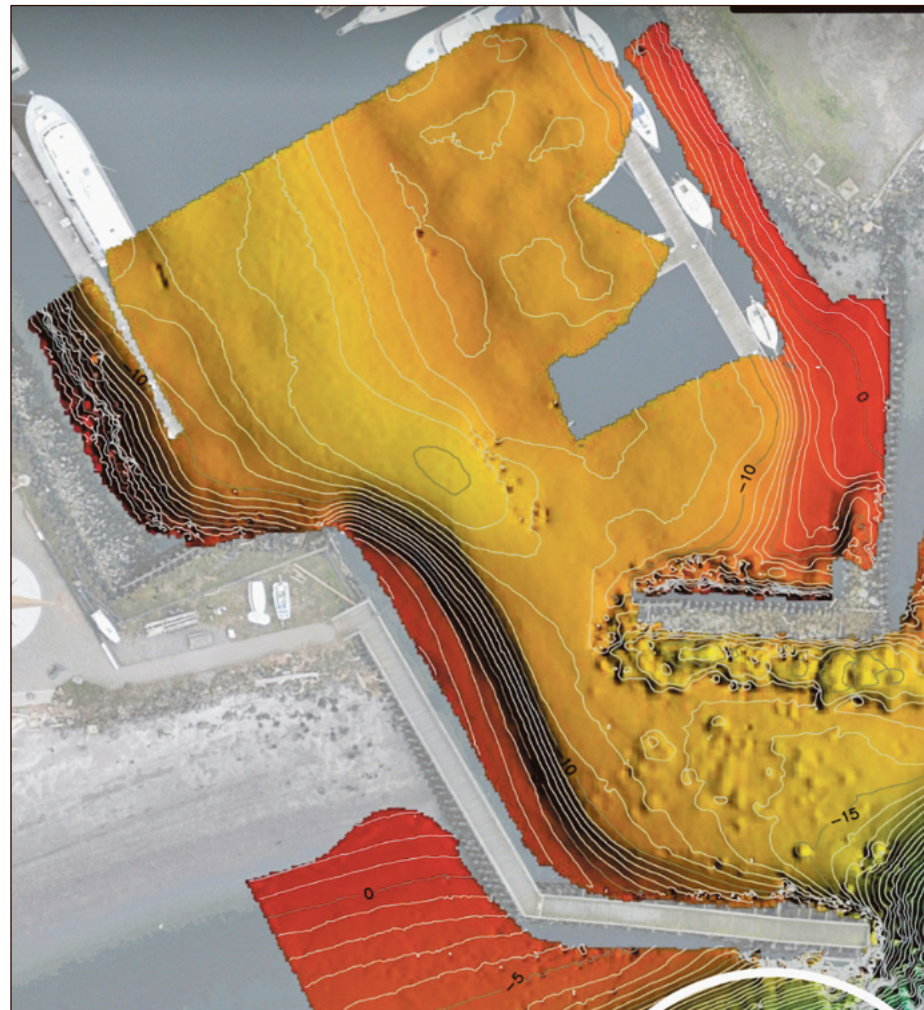
This schematic shows the location of the new, artificial reef, circled in white, just outside the Point Hudson South Jetty. The jetties are shown in grey; water depth is shown in color with red as the most shallow and blue as the deepest.
