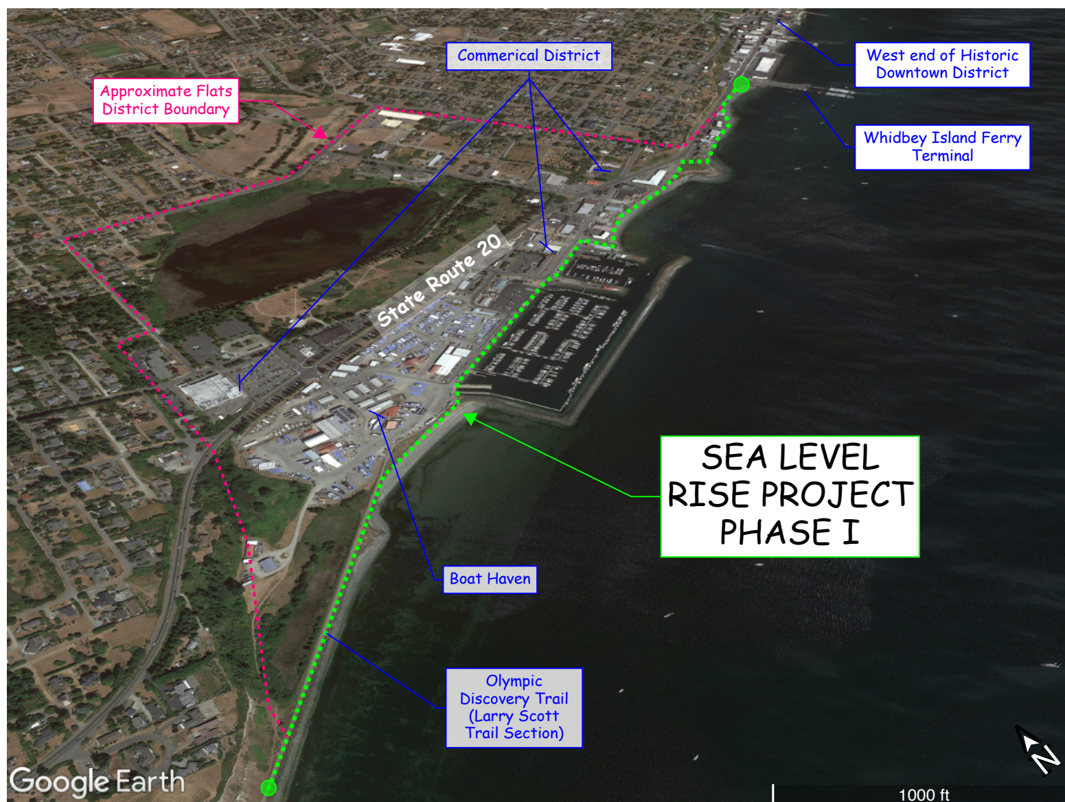
This schematic shows the outlines of the Sea Level Rise project, including the possible route of flood protection (green line) and the preliminary boundary of the low-lying Flats District (pink line). The flood protection would reach from two geographical high points.
