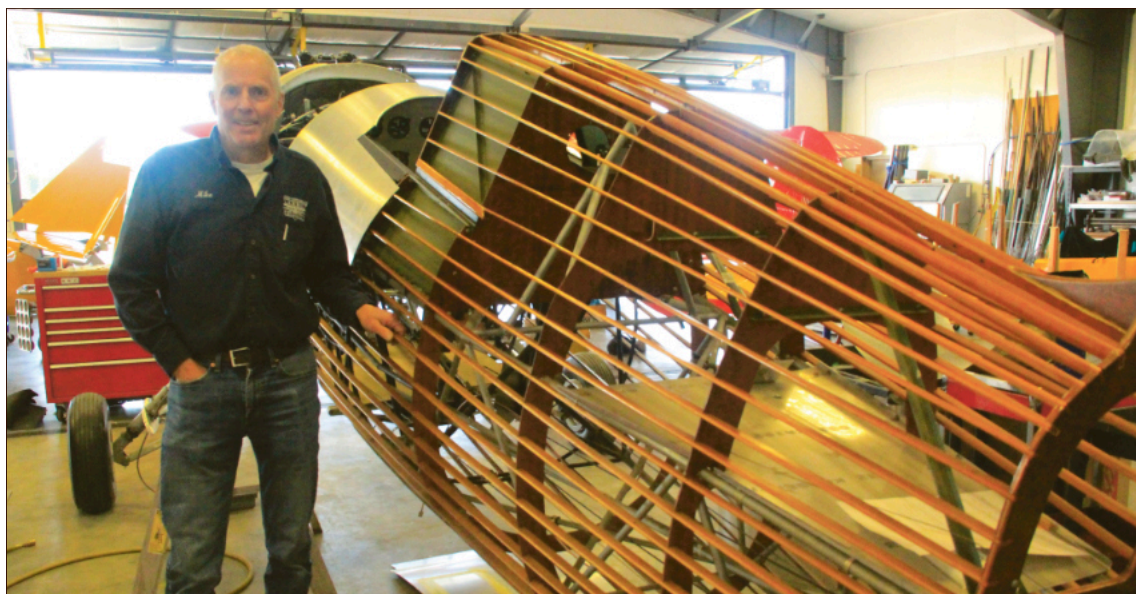
Michael Payne stands in front of the spruce framing of a World War II-era trainer airplane made by the Waco Aircraft Company. A private customer contracted the Aero Museum to do a complete restoration. The airplane had been stored for 40 years prior.
