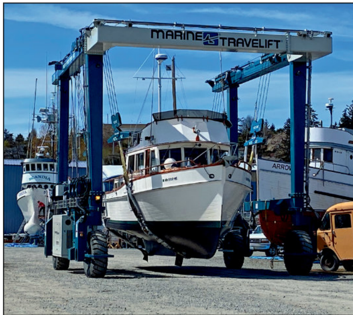
The Port owns and operates four Travelifts that carry vessels of up to 300 tons. In 2022 the Port bought a new 70-ton lift and did extensive maintenance work on the 300-ton lift. The Port earns money from haulouts and on-the-ground storage of boats.
