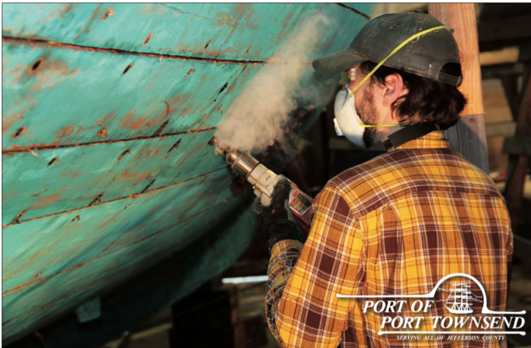
Gordon Kwiatkowski of Haven Boatworks looks through his drill bit's smoke and steam while refastening the hull of MV Carmelita.
