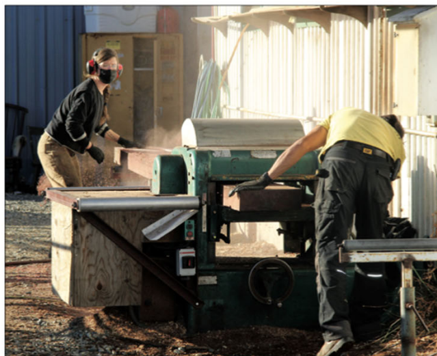
Claire Ethier and Chris Chimenti run purpleheart through Haven's thickness planer. It will become a transom guard on the MV Delight.
